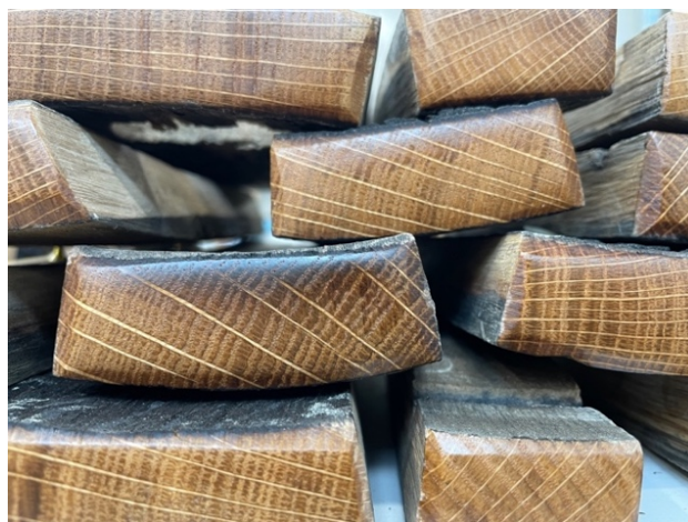
Fig. 12 The revealing of the medullary rays of oak trees. Whisky oak staves sanded with several sandpaper grades then oiled.
